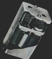
FIXED-TUNED EXCITER TANK
